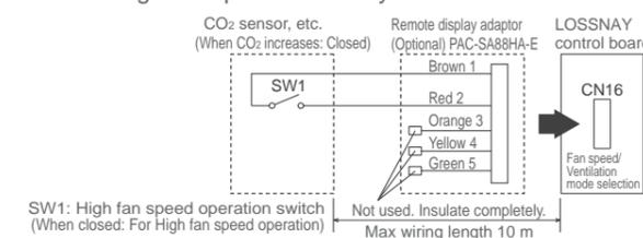
When SW1 is "ON", fan speed of the LOSSNAY will be set to "High"(Extra-High) regardless of the remote control setting. Use this in such a way that it ventilates at Low or Extra-Low fan speed normally, and when the external sensor detects contamination of indoor air, it changes to High (Extra High) fan speed operation.
