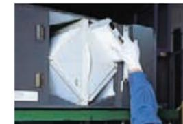
Incorporation into the main unit is simple, and filter changes can be performed via the main unit inspection opening.
