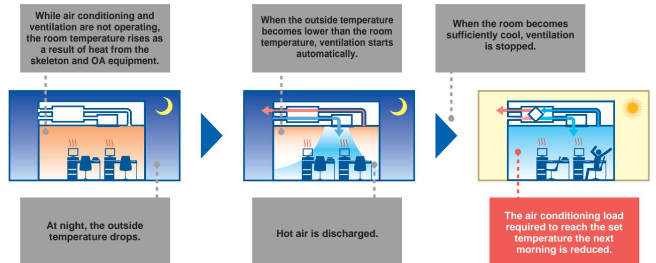
The out door temperature (OA) setting can be selected either 17°C or 28°C by using Dip-Switch (SW2-7) in the LOSSNAY control box. Refer to the Installation Manual for more information. \*Do not use the night purge function if fog and heavy rain is expected. The entry of rain water may occur in the night.
